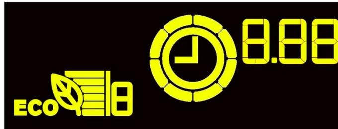
The Time Manager is represented on the right-hand side of the LCD display, and it consists of: eight segments surrounding the clock and three digits, which indicate the duration of the washing cycle.
