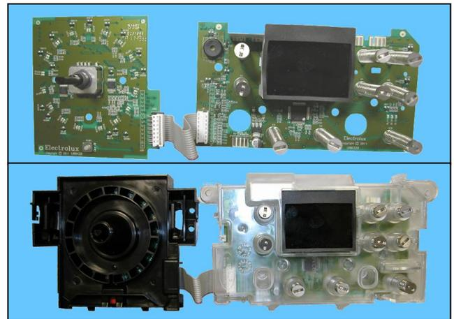
↗ The main circuit board is positioned at the rear of the appliance and receives commands from the display board, powers the electrical components as well as communicating with the motor control board (Inverter).
